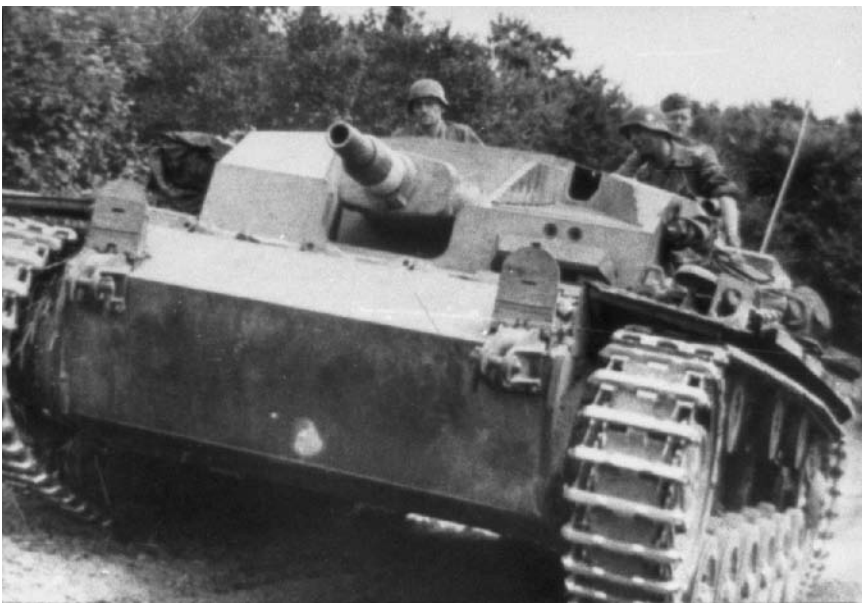
A StuG assault gun. Built on a Pz Mk III chassis and relatively easy to manufacture, this type of assault gun was used extensively by the Germans during the Ardennes offensive and was often quite successful, especially in an infantry support role (U.S. National Archives).
